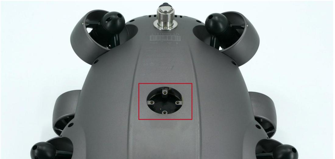
2. Place the Metal Detector directly at the bottom of ROV
